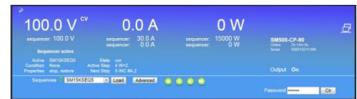
fig 7 - 2 Sequencer console for selecting and controlling sequences.
