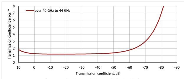
Specifications are based on matched DUT, and IF bandwidth of 10 Hz
