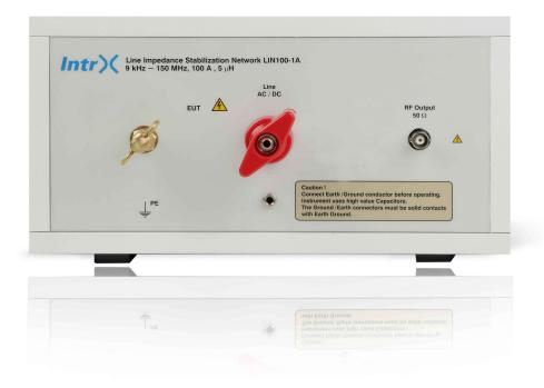
LISN (Artifical Mains Network) is a low-pass filter typically placed between an AC or DC power source and the EUT (Equipment Under Test) to create a known impedance as per complying standard for the measurement of conducted emission. It also isolates the unwanted RF signals from the power source with pre-filter included. It provides a Radio frequency (RF) noise measurement port.
