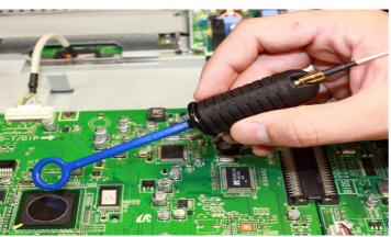
Pinpointing interference sources on a circuit board
