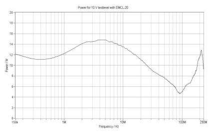
Measured amplifier output power to obtain a test level of 10 V. 6 dB attenuator and 80 % amplitude modulation depth are taken into account.
