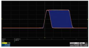
The rise/fall times can be set independently to the minimum of 16.8 ns at any frequency and to the maximum of 22.4 s. The adjustment step is as small as 100 ps. The Pulse width can be fine-tuned to the minimum of 32.6 ns with the adjustment step as small as 100 ps.
