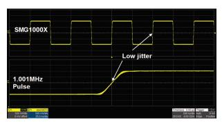
When a Pulse waveform is generated by a common DDS generator, there will be a one-clock-jitter if the sampling rate is not an integer-related multiple of the output frequency. SMG1000X Easy Pulse technology successfully overcomes this weakness in DDS designs and helps to produce low jitter Pulse waveforms.
