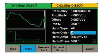
Up to 10 harmonics may be generated. Amplitude and phase of each harmonic can be set independently
