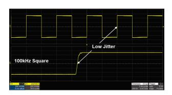
Benefitting from a special square-wave generating circuitry, the Square from the SMG1000X breaks the 60 MHz bandwidth barrier, reaching rise/fall times of less than 4.2 ns, and frequencies up to 60 MHz.
