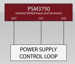
As illustrated above, the PSM3750 eliminates the requirement for an isolation transformer and differential probes. Another disadvantage when using conventional FRA instruments whilst performing analysis over a wide frequency band is that many different isolation transformers will be required for the different frequency ranges of the test. The PSM3750 eliminates this problem and generates frequencies throughout its entire frequency range from a single output.
