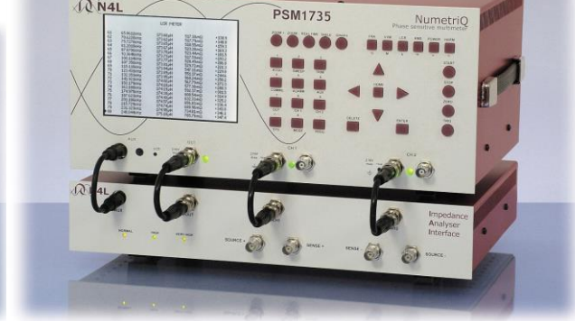
PSM1735 with Impedance Analyser Interface
