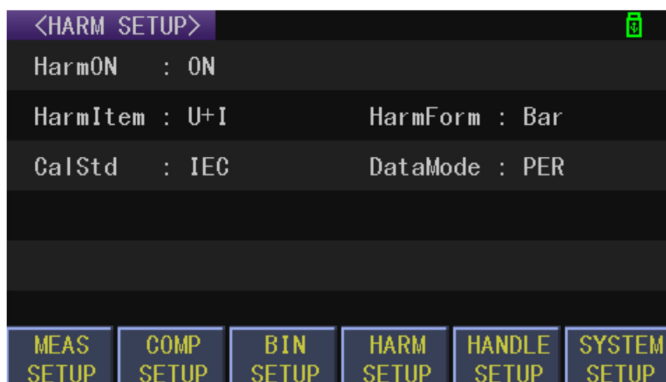
Figure 4-17 Harmonic setup interface
