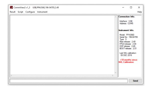
When connecting to the instrument the panel to the right hand side of the software window will display details about the instrument.
