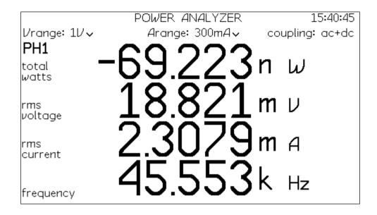
**REAL-TIME** toggles between continuous display readings and holding an instantaneous reading on screen. *Note: measurements continue to be taken even when display is in Hold.*
