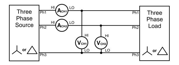
Three Phase-Three Wattmeter - simulated neutral
