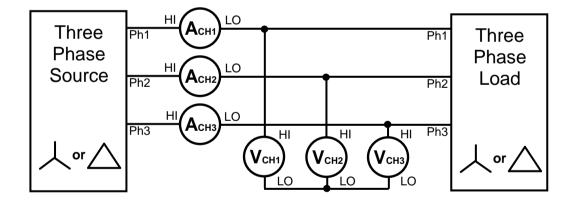
Three Phase Three Wattmeter – Star Connections
