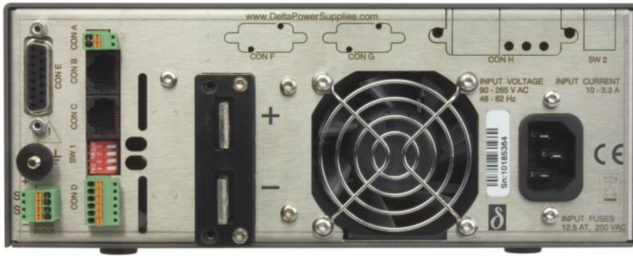
fig 3 – 8 Location of output terminals and analog programming connector on the rear panel.
