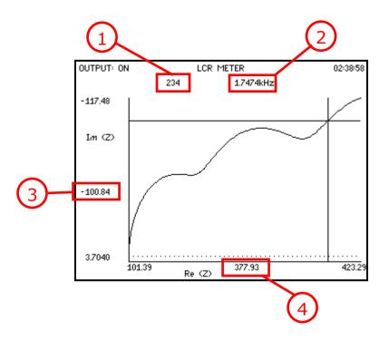
The axes are scaled to fit the sweep and a cursor is automatically displayed. The directional keys on the PSM's front panel can be used to navigate the cursor.
