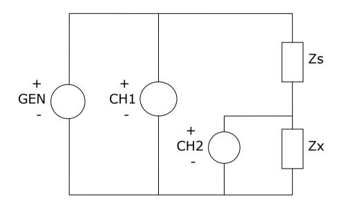
For "divider Zx low" connection, shown above, the total voltage is measured by CH1 and the voltage arising from the potential divider effect of Zs and Zx is measured by CH2. Notice that all the negative terminals are connected together.
