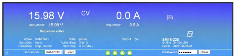
fig. 7 - 2 Sequencer console for selecting and controlling sequences.
