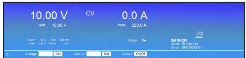
fig. 7 - 1 Front console for setting of the output and monitoring various parameters.
