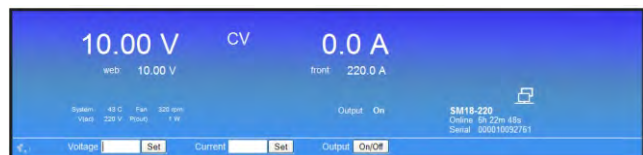
fig. 3 - 5, The front console of the web interface for setting of the input and monitoring various parameters.
