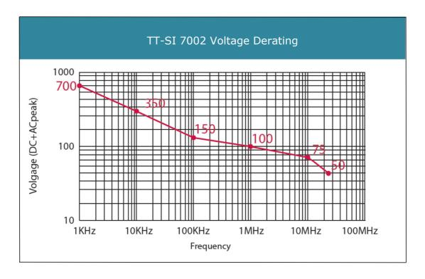
Figure: TT-SI 7002 Derating Curve
