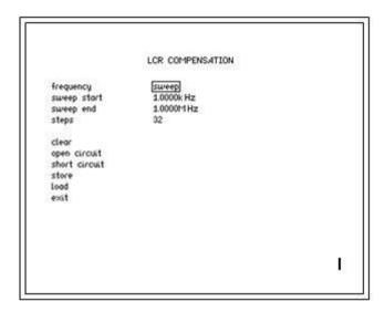
Here, the ZERO key has been pressed on the PSM front panel to present the LCR Compensation screen and then by using the navigation keys, the frequency option has been changed form 'single' to 'sweep'.
