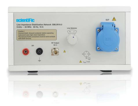
LISN (Artifical Mains Network) is a low-pass filter typically placed between an AC or DC power source and the EUT (Equipment Under Test) to create a known impedance as per complying standard for the measurement of conducted emission. It also isolates the unwanted RF signals from the power source with pre-filter included. It provides a Radio frequency (RF) noise measurement port.
