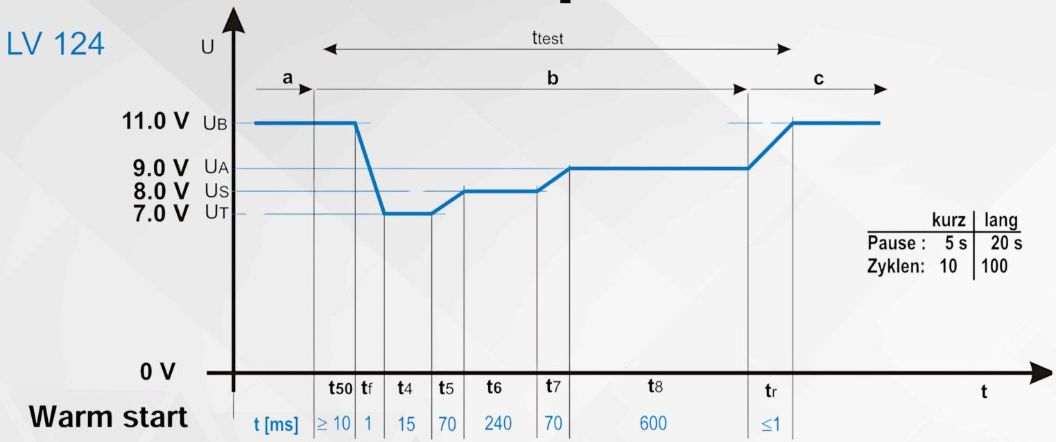
At test case 2 warm start (automatic restart after a stop),
