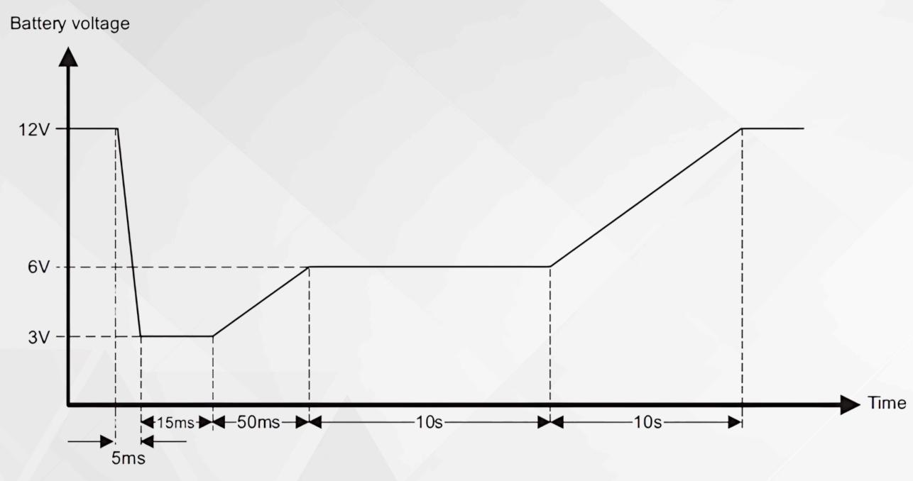
Figure 1. Typical Battery Voltage Profile Under a Cold-Cranking Condition
