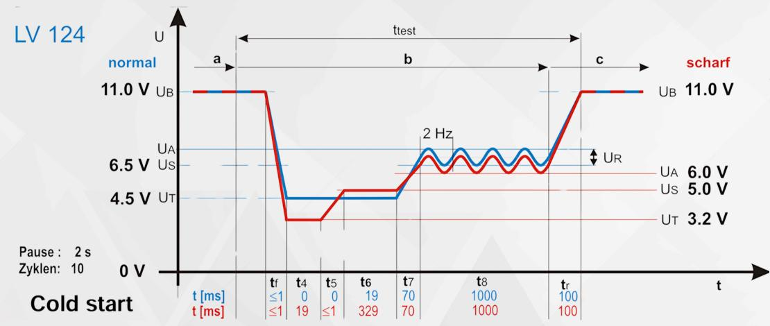
At test case 1 cold start (start the engine), there are test impulses for:
