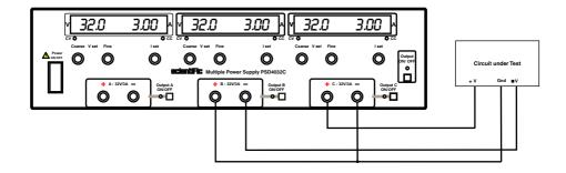
Note : The Value +V & -V will be as per set output voltage & current on power supply A & B individually.
