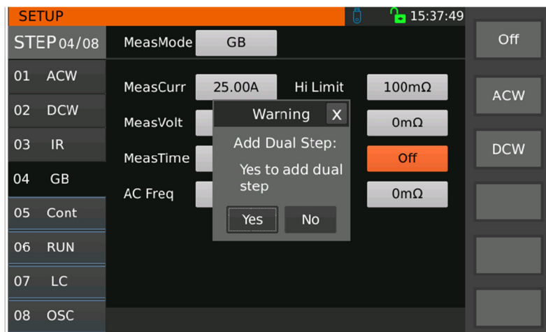
Figure 3-23 Simultaneous testing of grounding resistance and AC withstand voltage
