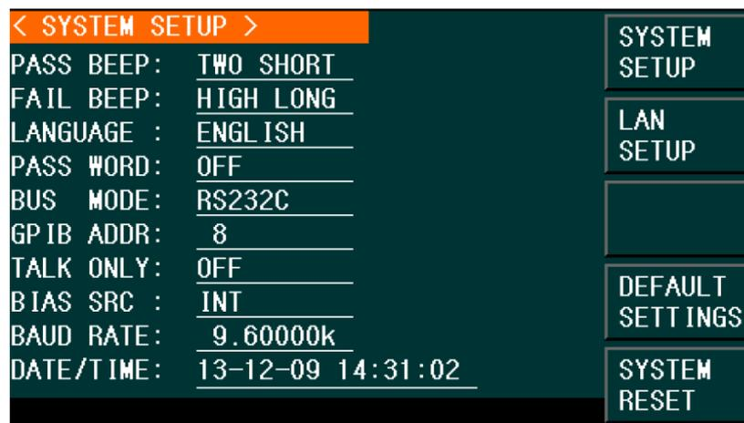
On this page, most system setup items are displayed, such as instrument main function, beeper, PASS beeper, FAIL beeper, language, PASS word, bus mode, GPIB address, TALK only, Bias SRC, baud rate, data/time.
