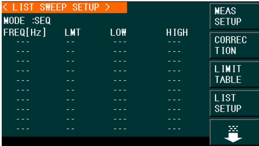
The list sweep function of SM6025 can perform auto sweep test for the test frequency, test level or bias voltage of 10 points. On <LIST SWEEP SETUP> page, the following list sweep parameters can be set.
