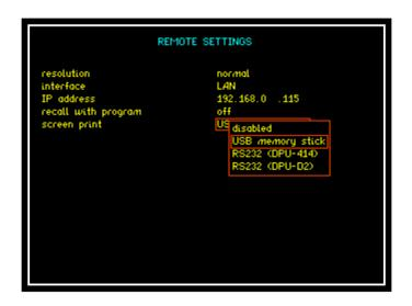
By default the save location for the screen shot will be the USB memory stick; this can be changed in the 'Remote' menu. You can change it to print to the RS232 port, that is used to print to an attached printer to print a physical copy of what is shown on the screen described in 6.4.
