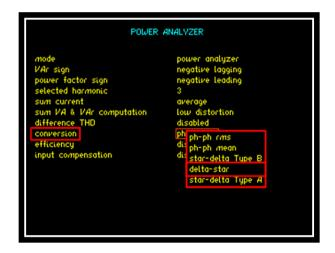
It is not possible for the instrument to detect the wiring configuration used to connect the instrument to the motor / DUT. All "conversion" options have to be available with the User ensuring the correct option is selected from the menu.
