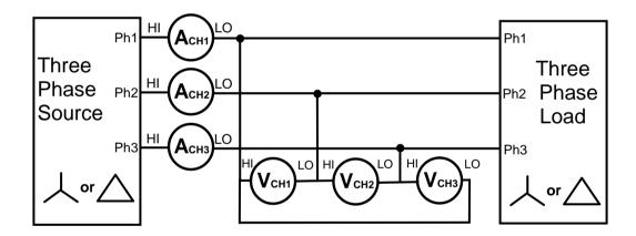
On a multi phase instrument, all the phases usually use the same input control data – internal/external, scaling factor etc. It is possible to select "independent" so that the phases can be set up differently. This is useful if different scaling factors are required for external shunts or if one phase is using internal shunt when others are external.
