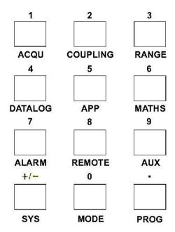
**SELECT MENUS** for non mode-specific configuration. Also, use as numeric keypad when entering parameter values or data.
