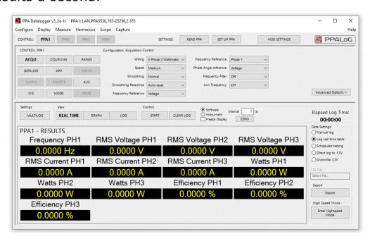
Measure mode is a truly flexible measuring system which will fulfil most needs. The Parameters to be datalogged are selected using the Multilog selection window:
