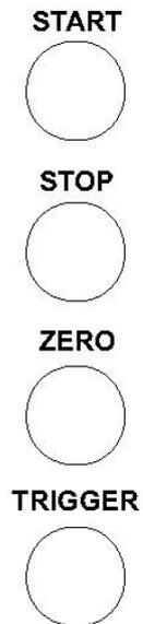
**START** & **STOP** datalog function (when enabled) or integration (*Integ* mode). Either key also triggers single-shot in *Scope* mode.
