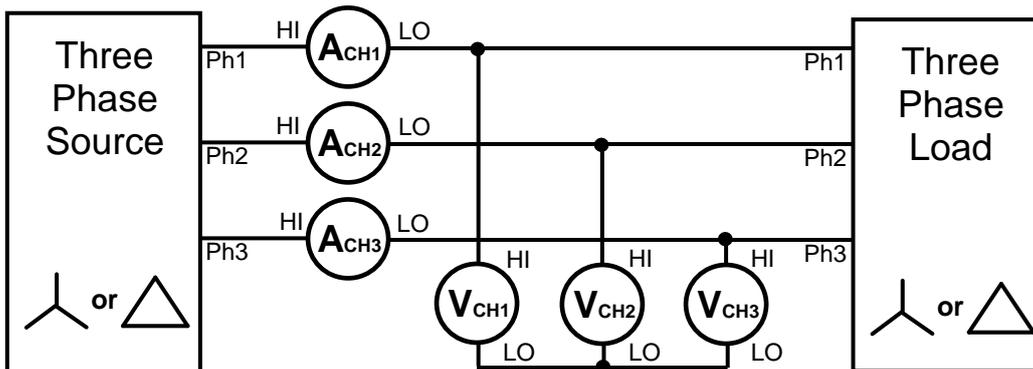
Three Phase Three Wattmeter – Star Connections
