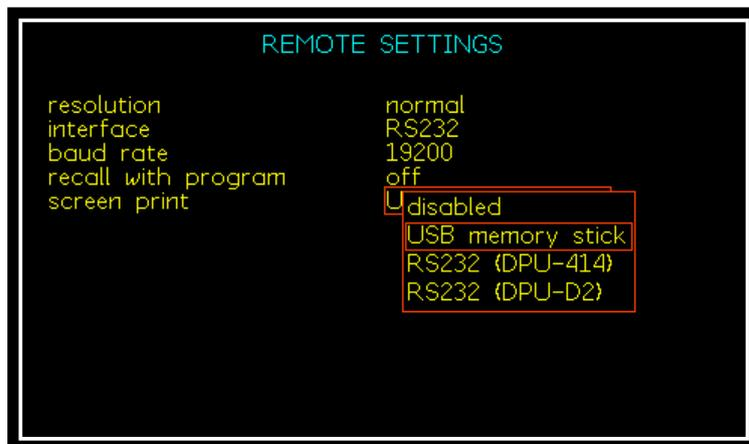
The "active" side of the display will be printed; for both sides press NEXT or BACK to switch to the other side and hold START again.
