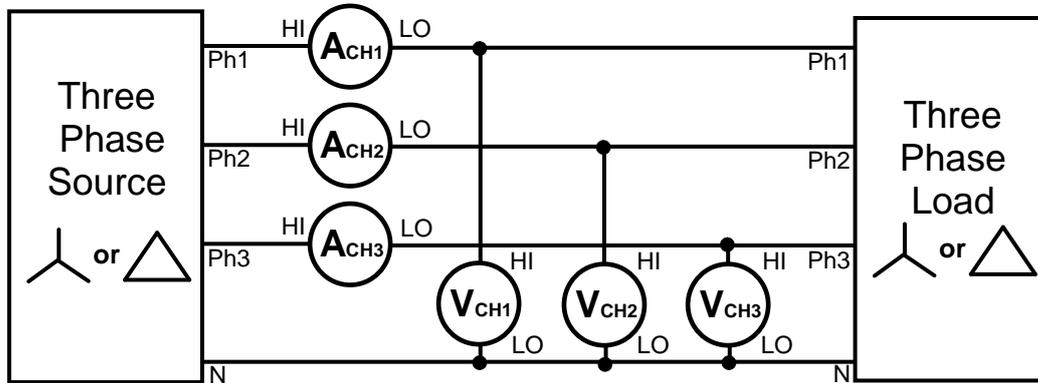
To configure PPA35xx to calculate the correct phase power when the Load topology is in a Star Configuration:
