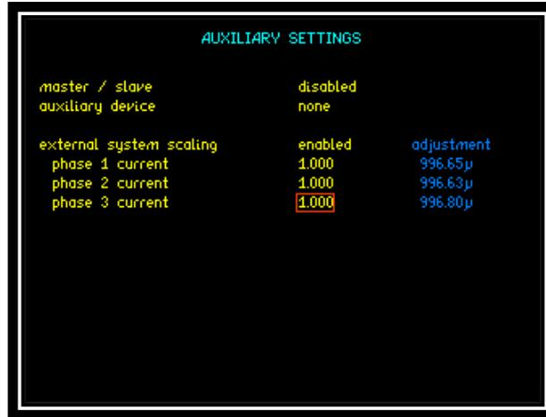
Pressing the RANGE key to display the RANGING menu will confirm that the external system scaling has been selected in the AUX menu. The Scale factor and the nominal shunt value will be displayed in green text. The screenshot below shows the settings for Phase 1.
