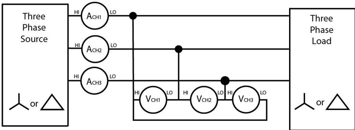
To configure PPA35xx to calculate the correct phase power when the Load topology is in a Delta Configuration:
