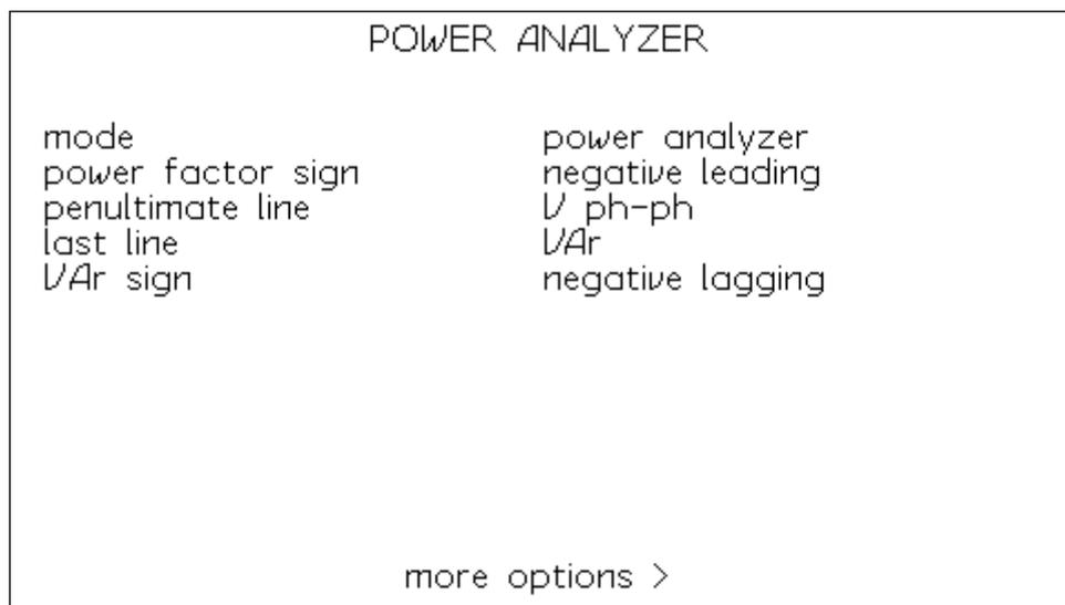
Use UP and DOWN keys to highlight an option, and ENTER to confirm (see para. 3.3 Menu Control Keys). Parameter values within the selected option may be adjusted using the L or R keys or by entering a numeric value directly, as indicated. Press ENTER to confirm.
