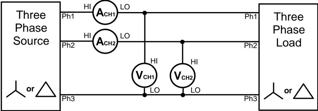
Three Phase Three Wattmeter - simulated neutral
