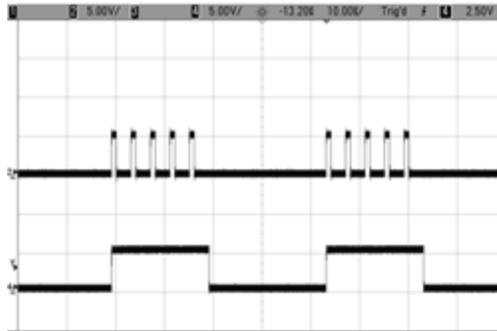
**Inhibit Mode** – Channel H is used to inhibit the output of the selected channel(s). This is an active high pulse, thus when channel H is high the selected channel(s) will **NOT** output pulses.
