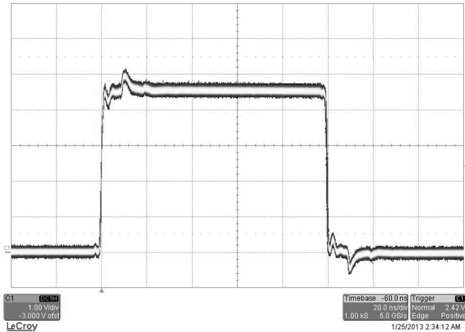
Figure D.1 – TZ50 Option Into 50 Ohm Load
