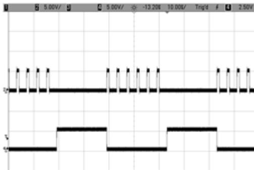
**Invert Mode** – Channel H is used to invert the output of the selected channel(s). This is an active high pulse, thus when channel H is high the selected channel(s) will be inverted
