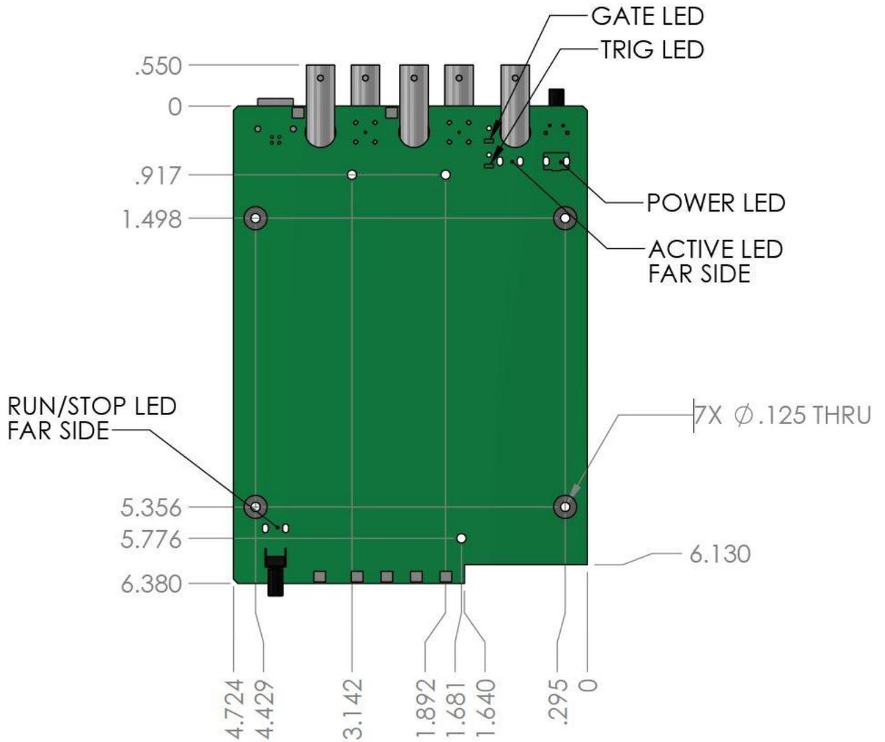
Figure 15-2 Mechanical Dimensions
