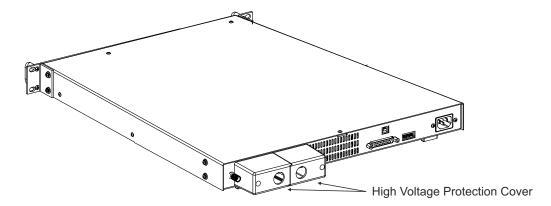
Mounting of this part is very simple. Pass the cables through the protection cover before mounting the cables on bus bar. Connect the cables on bus bar, push the protection cover to touch the rear panel and fix with the screws.
