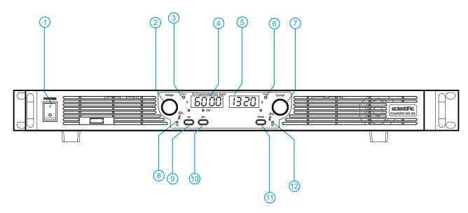
1 AC Power Switch: Mains AC power ON/Off control, when switched to ON, supplies main AC power
