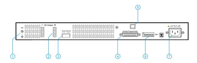
1) PE : Terminal provided to make connection to protective earth.
