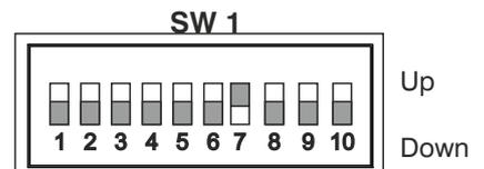
Switch SW1 set for both voltage and current remote programming, DIP switch 7 & 9 moved up.
