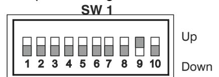
Rear panel switch SW1 set for remote external current programming, when DIP switch 7 is moved up. Voltage setting is from front panel.
