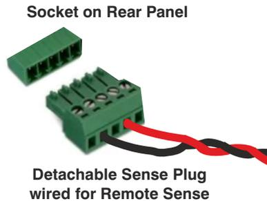
If the voltage regulation is to be maintained at load point, external wires are to be connected to sense points. Connect the wiring as shown above in the plug and insert the plug in remote sense socket. Before detaching or connecting the sense wires, switch off the power supply output, and ac mains to the unit. Wait for two minutes, until the output get discharged.
