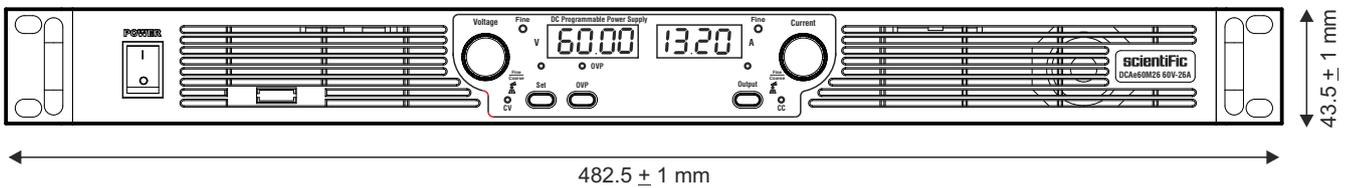
Note : When the power supply unit is mounted in 19" rack cabinet, instrument feet are removed and side rack mounting handle assemblies are fitted on both side.
