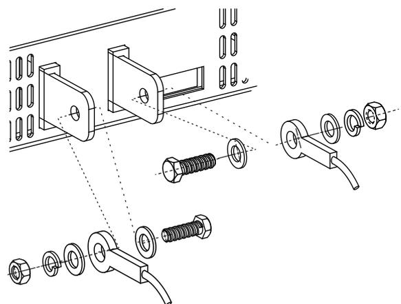
Ensure that the output cable/ wire connected on output terminal are securely tightened before applying the power.
