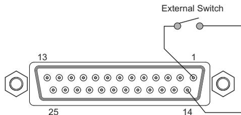
Pin 2 , Pin 3 , Pin 12, Pin 22, Pin 23 : Ground Analog Programming.
