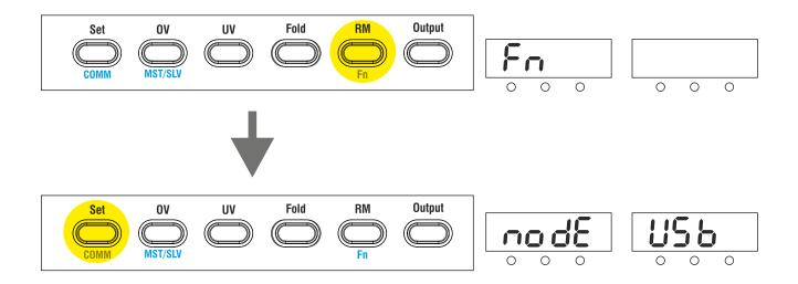
By varying voltage encoder you can select mode, baud and address.
