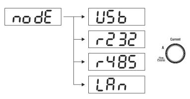
By varying current encoder baud parameters can be changed from 1200,2400, 4800, 9600 and 19.2k when baud is selected.
