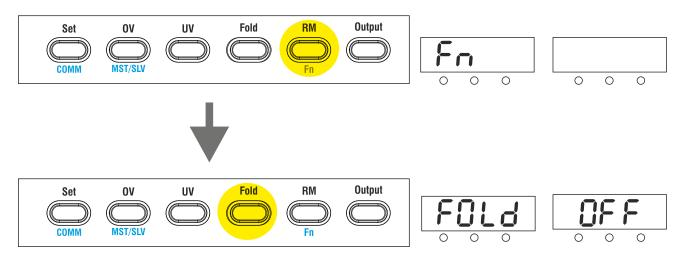
By varying current encoder mode, Fold function in CV or CC mode is selected. To switch off the Fold, select "Off".
