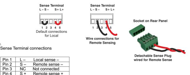
If the voltage regulation is to be maintained at load point, external wires are to be connected to sense points. Connect the wiring as shown above in the plug and insert the plug in remote sense socket. Before detaching or connecting the sense wires, switch off the power supply output, and ac mains to the unit. Wait for two minutes, until the output get discharged.
