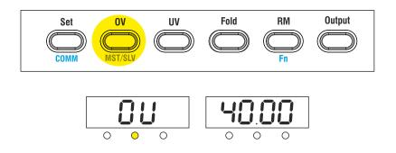
To set the new over voltage protraction value, rotate voltage encoder. The new changing value is displayed on right window. You can change the encoder resolution in coarse, medium or fine by pressing voltage encoder switch.
