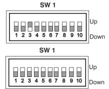
To disable the output or to keep the output OFF on mains AC switch ON, keep the switch 4 to down.
