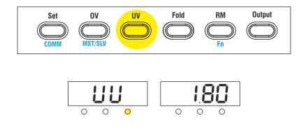
To set the new under voltage limit value, rotate voltage encoder. The new changing value is display on right window. You can change the encoder resolution in coarse, medium or fine by pressing voltage encoder switch. The maximum under voltage can be set to approx. 95 % the set voltage. The minimum under voltage value can be set to 0 V.
