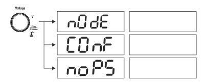
Once the mode or configuration or number of power supply units, their respective parameters can be set with the help of current encoder.
