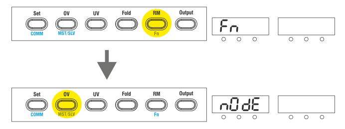
By varying voltage encoder you can select Mode, Configuration or number of power supply units.
