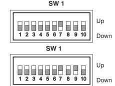
Switch SW1 set for both voltage and current remote programming, DIP
