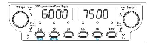
The front panel controls are ergonomically arranged to ease in operation. Apart from the two encoders on either sides named as Voltage and Current are used to select the modes and parameters, while in Menu selection.
