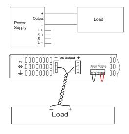
points, the sense wires are connected across the load.
