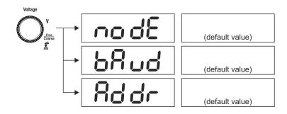
By varying current encoder mode parameters can be changed when mode is selected, from USB, Rs232, RS485 & LAN.
