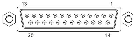
The Analog input output connector is D type 25 pin Female connector. Use appropriate mating connector always to give firm contacts and reliable connections.
