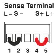
The five pin sense plug can be pulled out from the socket, place the wires and re-insert the plug in sense terminal socket.
