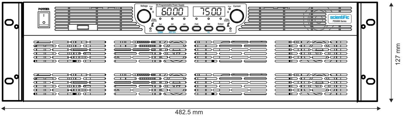
Note : When the power supply unit is mounted in 19" rack cabinet, instrument feet are removed and side rack mounting handle assemblies are fitted on both side.
