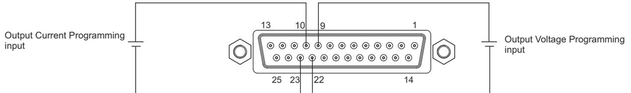
**Pin 11 : Voltage monitoring output ; Pin 24 : Current monitoring output**
