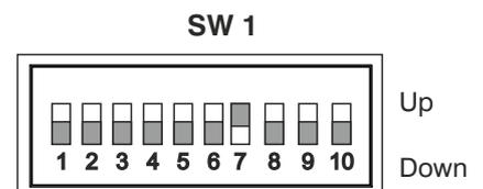
Switch SW1 set for both voltage and current remote programming, DIP switch 7 & 9 moved up.
