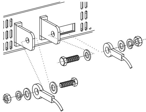
Ensure that the output cable/ wire connected on output terminal are securely tightened before applying the power.
