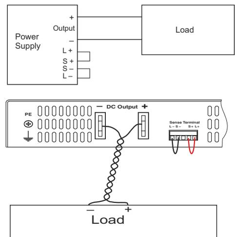
points, the sense wires are connected across the load.
