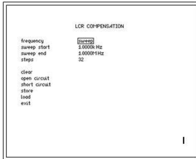
Here, the ZERO key has been pressed on the PSM front panel to present the LCR Compensation screen and then by using the navigation keys, the frequency option has been changed from 'single' to 'sweep'.
