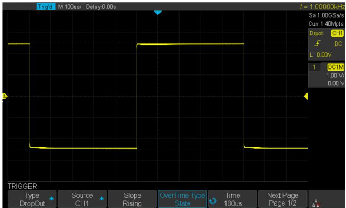
Figure 39 State DropOut Trigger
