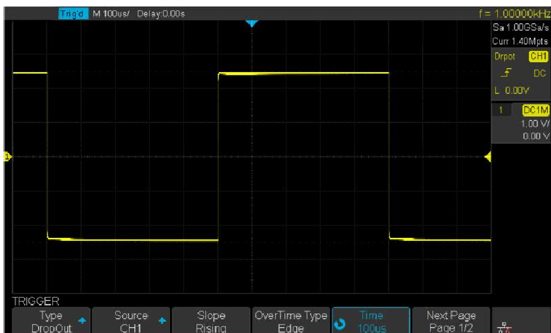
Figure 38 Edge DropOut Trigger
