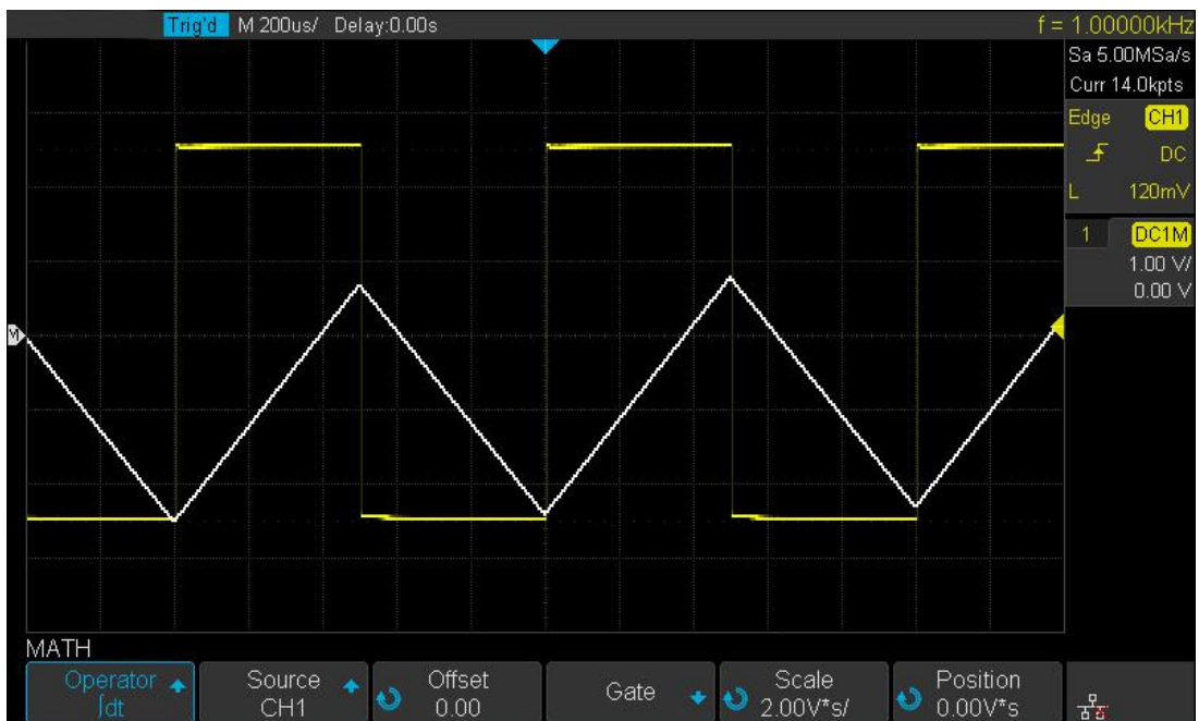
Figure 84 Integral with Offset
