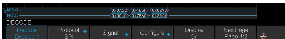
Figure 52 SPI Decode Bus Display
