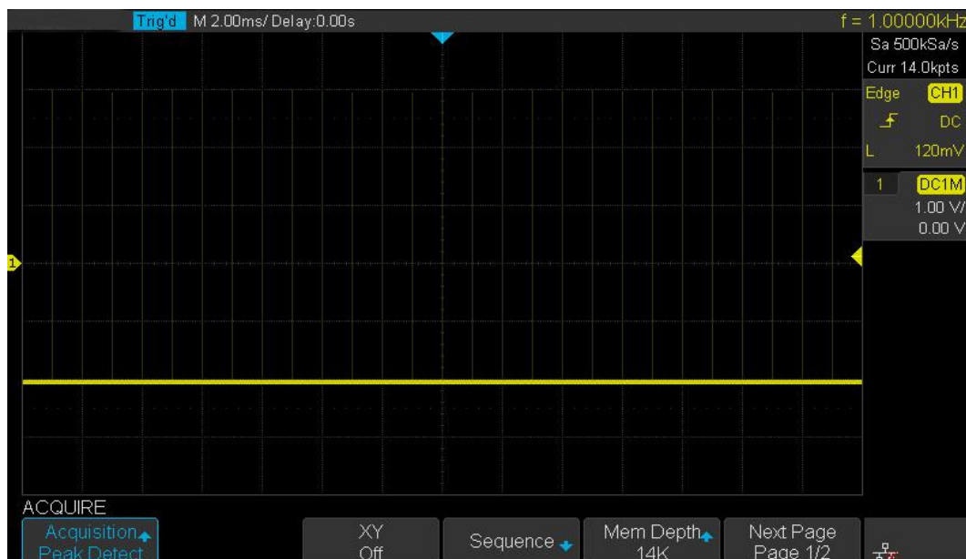
Figure 24 Pulse With 0.1% Duty, Peak Detect Mode
