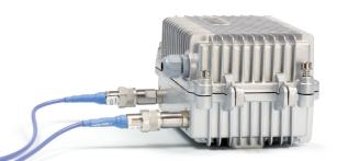
Pictured here is an TR1300 VNA testing a 50  $\Omega$  amplifier.
