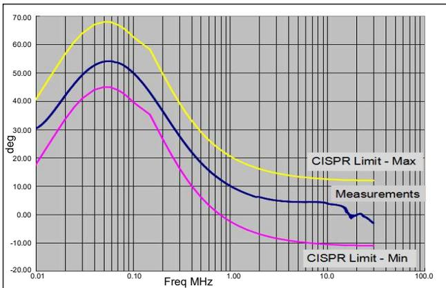
Isolation curve Terminal EUT RF
