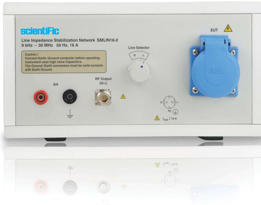
LISN (Artificial Mains Network) is a low-pass filter typically placed between an AC or DC power source and the EUT (Equipment Under Test) to create a known impedance as per complying standard for the measurement of conducted emission. It also isolates the unwanted RF signals from the power source with pre-filter included. It provides a Radio frequency (RF) noise measurement port.
