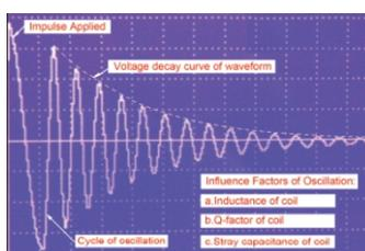
The Decay curve of winding voltage
