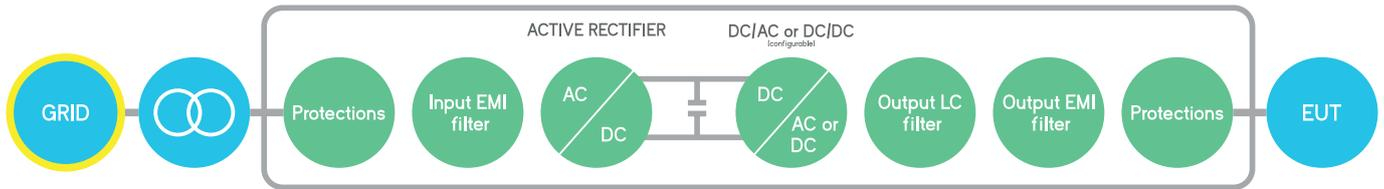
The hardware platform is based on a Back-to-Back power conversion topology, formed by two IGBT-based power stages. The grid side stage is an Active Rectifier which produces clean sinusoidal currents with very low harmonic distortion and power factor close to one.
