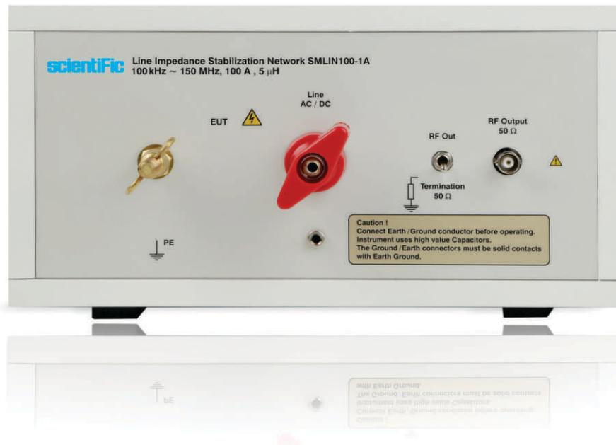
LISN (Artificial Mains Network) is a low-pass filter typically placed between an AC or DC power source and the EUT (Equipment Under Test) to create a known impedance as per complying standard for the measurement of conducted emission. It also isolates the unwanted RF signals from the power source with pre-filter included. It provides a Radio frequency (RF) noise measurement port.
