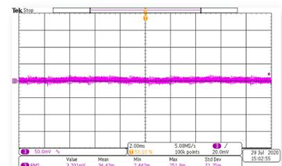
Voltage ripple on DC output with DBx Module<sup>1</sup>
