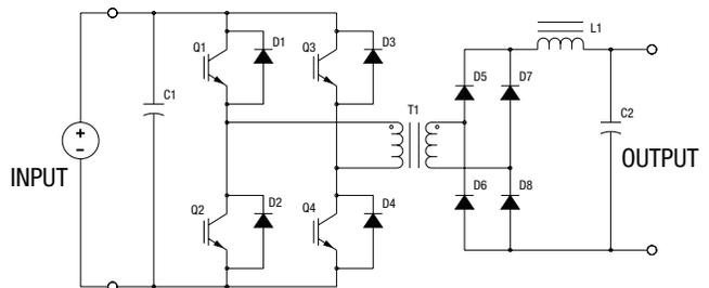
Figure 1. Voltage-Fed Converter
