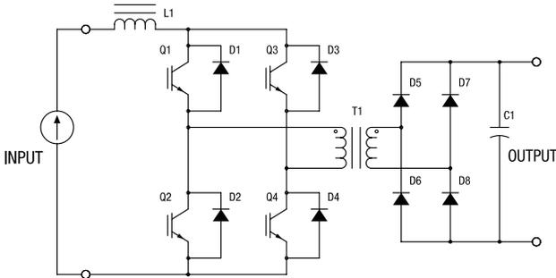
All MagnaDC programmable DC power supplies utilize high-frequency IGBT-based power processing in current-fed topology. This topology adds an additional stage over the conventional voltage-fed topology for enhanced control and system protection, ensuring that even under a fault condition, the power supply will self-protect. Due to the self-protecting characteristics of this topology, the possibility of fast rising current spikes and magnetic core saturation is eliminated.
