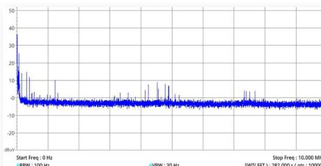
Common mode noise on DC output with DBx Module<sup>1</sup>
