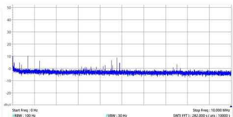
Differential mode noise on DC output with DBx Module<sup>1</sup>
