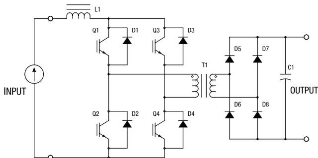
Figure 2. Current-Fed Converter
