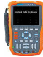
Handheld DSO 60-200MHz, Dual Isolated Channels RTS 1GSa/s, Memory upto 1Mpts Built in DMM
